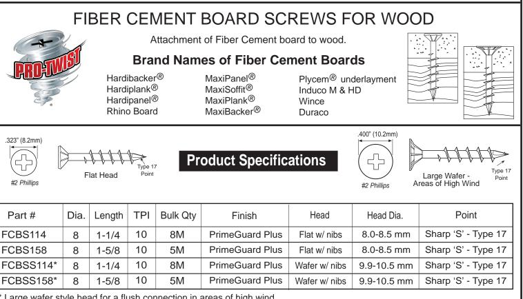
\* Large wafer style head for a flush connection in areas of high wind.
